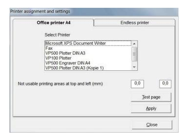
Now choose the printer you require and click on the button **Test page**. A **< Portrait test page >** sheet is then printed on the relevant printer. Measure the top and left margin with a ruler and enter the values in the respective boxes. These entries are needed because all printers have different margin settings for text.
