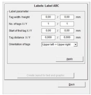
The sequence for labeling can be either from upper left > to upper right (line by line), or from upper left > to lower left (column by column).
