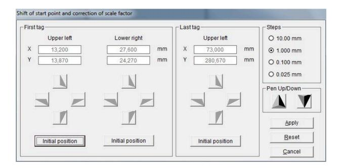
Insert a plotter pen into the pen holder or the optical measurement tool with hairline cross into the engraving head (spindle location) and click on the button **Initial Position** in the far left field.
