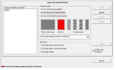
If you have a plotter with support plate recognition, it is advisable to use this function to make it easier later on to find the marking element that you have created. To do this, the plotter must be switched on and the relevant support plate positioned on the plotter.
