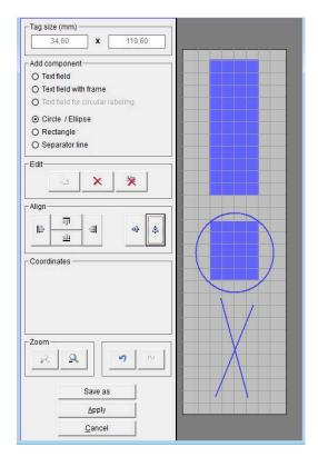
Click on the **Apply** button to apply the layout to the previously selected tags. You can now enter labeling data straight into the fields.
