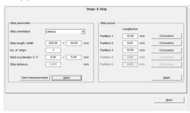
By using the < **Take measurements** > function, it is easy to calculate the start coordinates and the strip spacing.
